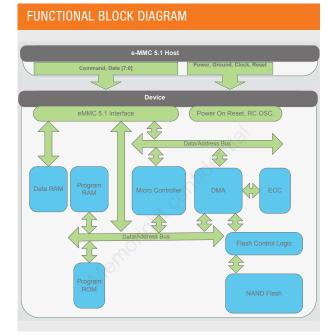
up to 32 GB storage capacity that makes it an ideal solution for multimedia handsets. M1890 integrates advanced flash management technology to achieve balance between cost and performance. It supports three clock frequency of 0-200 MHz and also supports for data bus width modes of 1 bit, 4 bit and 8 bit. Besides, it integrates several patented method such as dynamic & static wear-leveling and advance block management to achieve highest data reliability and maximized flash life expectancy.
