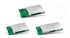
Panasonic expand their product line with WLAN / Wi-Fi modules. These operate in the 2.4 GHz ISM band and enable rapid wireless implementation in a variety of applications. With an excellent 802.11 wireless radio and baseband processor in a system-on-chip (SoC) design achieves maximum WLAN performance.
