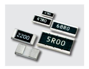
**The new Susumu high power thin film chip resistor** are designed to meet the high power rating that applications like inverter, DC motor driver or automotive electronics require. Being optimized for high power handling capability, PRG and HRG series bring also all the well known advantages of the thin film technology such as tight tolerance, excellent TCR, very high reliability and low current noise with them.
