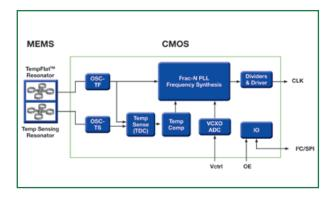
Elite is an innovative MEMS timing Platform for precision TCXOs, VCXOs, and low jitter oscillators.
