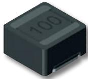
**For their QS series, ABC chose** square type ferrite cores instead of the commonly used round version which enables the total automatization of all process steps. This change enlarges the available space for the winding. The application of modern ferrite mixtures helps to further optimize all electronic performances, especially the Rdc, which leads to a reduction of total losses. By omitting the manual process steps, the production yield rate and quality are significantly increased.
