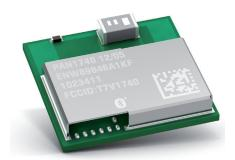
**PAN1740** is the next generation Bluetooth Low Energy Module from Panasonic with reduced form factor, significantly lower power consumption and embedded Software Stack.
