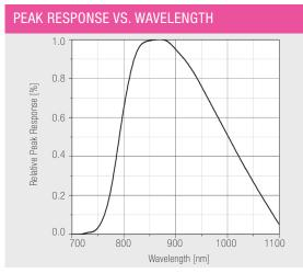
The **PTP83016BT24** is a silicon NPN phototransistor in SMD package. The device comes with a superior filtering for visible light by utilizing special black molding compound.
