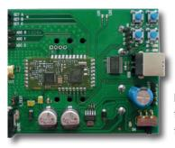
Evaluation board for testing the XTR-8LR100 transceiver performance.
