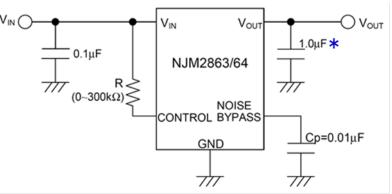
\* To manufacture, distribute and sell unit products using this product in the EU (European Union) accession, in order to comply with Conductive Emission (EN 55022 Class B), 22uF and more of capacitors is connected to this product's power input terminal (Pin 1: Vdd port).
