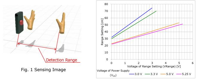
Fig. 2 Range Setting against Voltage
