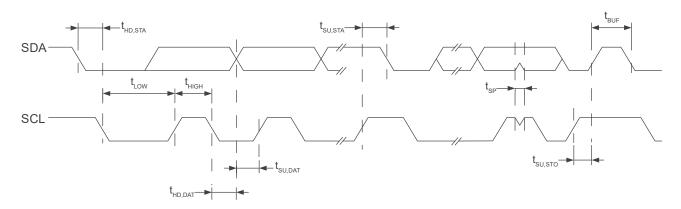
Figure 4.2: I<sup>2</sup>C Mode Timing Diagram
