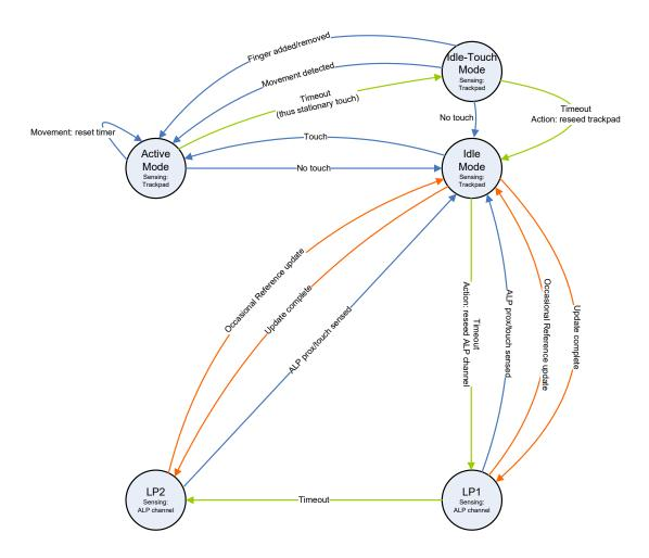
Figure 6.1: System Mode State Diagram
