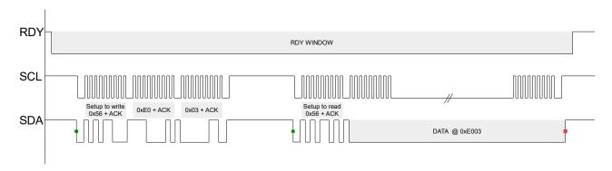
Figure 11.2: Extended Addressing Comms Diagram (Specific Channel)
