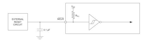
Figure 4.1: MCLR Pin Diagram
