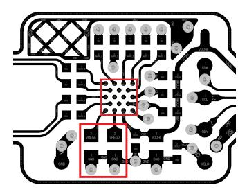
Figure 13.2: VREG Capacitor Placement Close to IC
