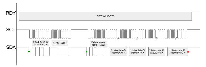
Figure 11.1: Extended Addressing Comms Diagram
