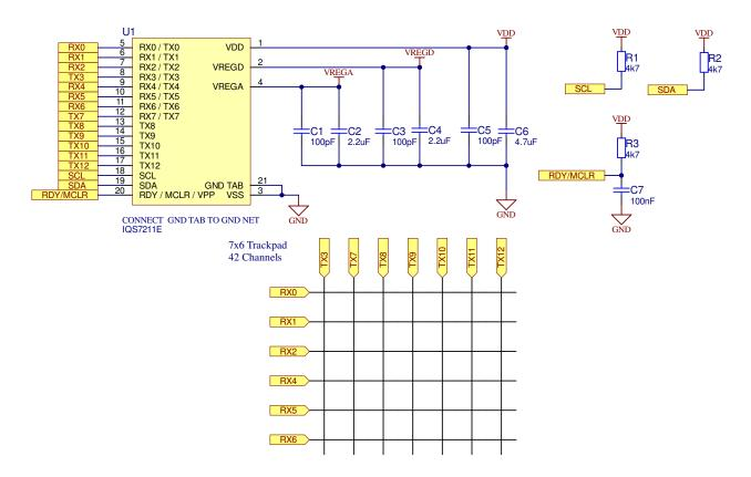
Figure 2.1: Reference Trackpad Schematic: 7x6 Pattern
