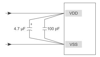
Figure 13.1: Recommended Power Supply Decoupling
