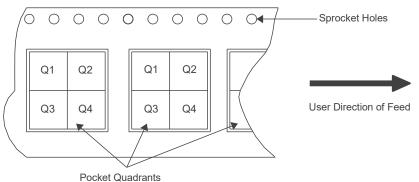
Figure 15.3: Tape and Reel Specification
