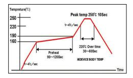
Recommended Peak Temperature : 250°C Max 250°C up /within 10secs Max. Reflow temperature : 260°C Gradient of temperature rise : av 1-4°C/sec Preheat : 160-190°C/within 90-120secs 220°C up /within 30-60secs Composition of solder Sn-3Ag-0.5Cu
