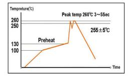
Solder bathtub temperature :  $260^{\circ}$ C max within 5secs. Preheating temperature :  $100 \sim 130^{\circ}$ C deposit solder temperature. Composition of solder Sn-3Ag-0.5Cu
