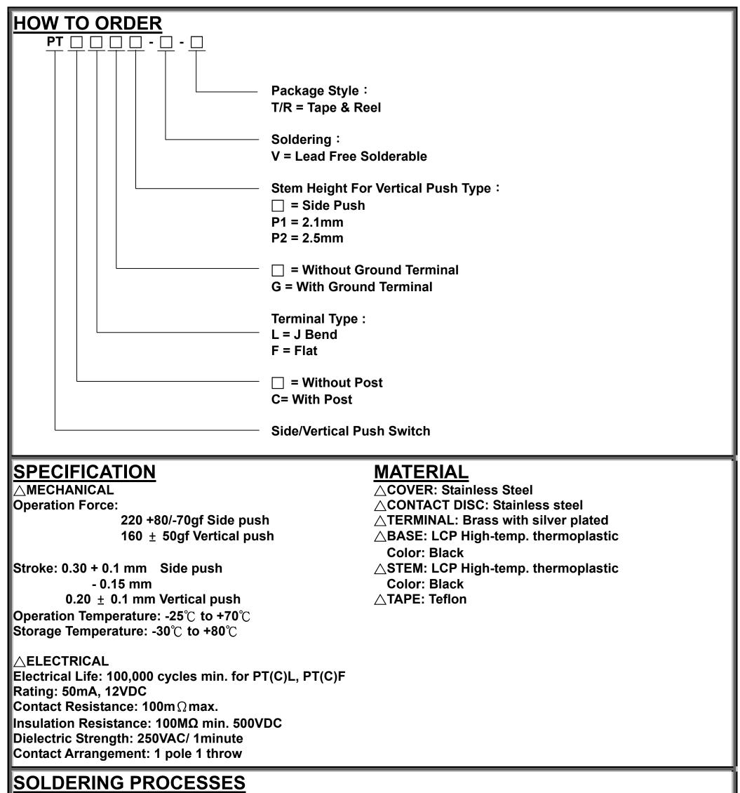
$\triangle$ HAND SOLDERING : Use a soldering iron of 30 watts, controlled at 350 $^\circ$ C approximately max 5 seconds.
