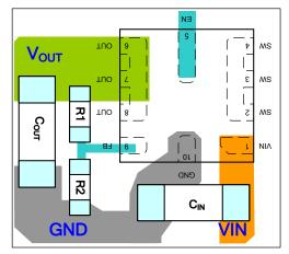
Figure 7: Single-Layer PCB Layout
