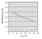
Figure 8: Maximum Output Current vs. Output Voltage
