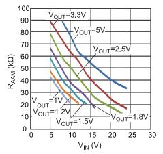
Figure 10. Recommended AAM Resistor Selection
