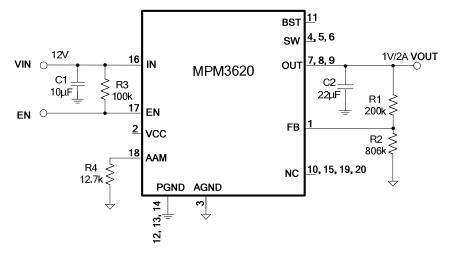
Figure 18. V<sub>OUT</sub>=1V, I<sub>OUT</sub>=2A
