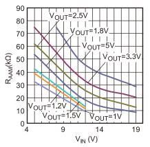
**Figure 7: AAM Resistor Selection**
