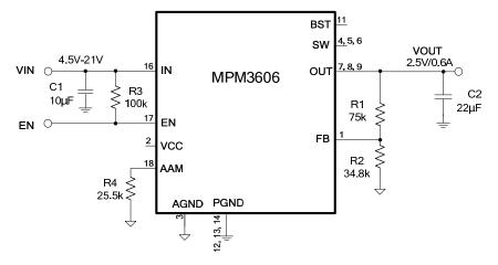
Figure 10: V<sub>OUT</sub>=2.5V, I<sub>OUT</sub>=0.6A
