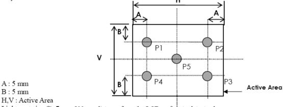
Light spot size ∅=7mm, 500mm distance from the LCD surface to detector lens measurement instrument is TOPCON's luminance meter BM-5
