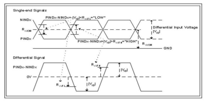
3. Input Clock And Timing Diagram
