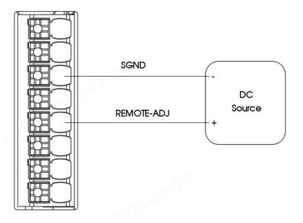
If the input end of the power module is connected to the power supply, the output voltage can be controlled within the specifications by using the external voltage (3V to 18V) between the REMOTE-ADJ signal pin and SGND, as shown in the figure.
