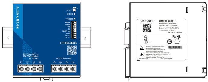
Note: Keep the following installation clearances: 40mm on top, 20mm on the bottom, 5mm on the left and right sides are recommended when the device is loaded permanently with more than 50% of the rated power. Increase this clearance to 15mm in case the adjacent device is a heat source (e.g. another power supply).
