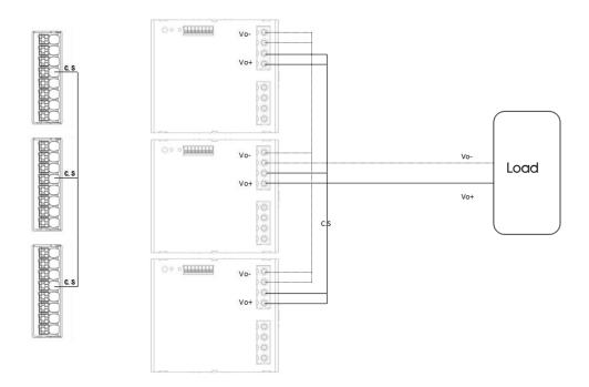
Note: 1. When used in parallel, the number of parallel modules cannot exceed 3.
