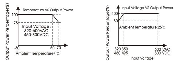
Note: 1. All curves are for 24V output, measured at input 3x400VAC, 50Hz, output Io, ambient temperature 25 °C, unless otherwise stated;
