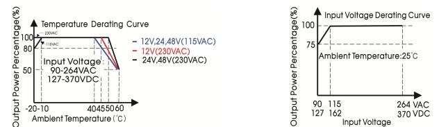
Note: 1.With an input voltage between 90 -115VAC and a DC input between 127-162VDC the output power must be derated as per the temperature derating curves;
