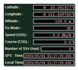
The **Navigation View** displays the primary navigation information, the units of measurements are determined in the Unit selection box.
