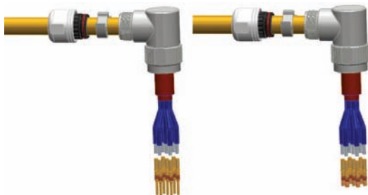
Step 7: Attach contacts to wire leads
