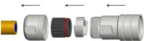
Step 1: Slide parts onto cable
