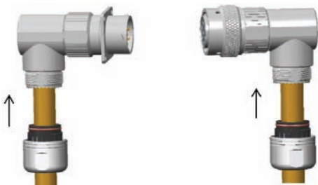
Step 11: Push shielding clip into backshell
