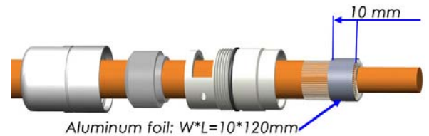
Step 4: Wrap foil over braided shielding
