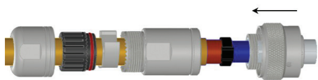
Step 6: Slide plug onto crimped terminal assembly
