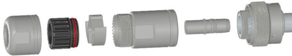
Step 2: Strip jacket to braided shielding and attach tie wrap
