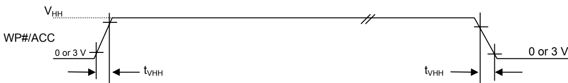
Figure 11. Accelerated Program Timing Diagram
