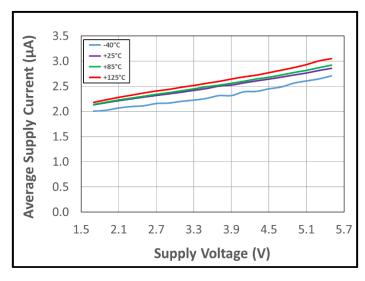
Figure 6. Average Supply Current vs. Supply Voltage vs. Temperature
