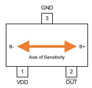
Figure 2. CT812x: 3-Lead SOT23 Package for Digital Output
