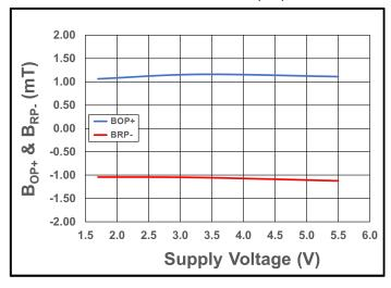
Figure 4.  $B_{OP+}$  (Blue) and  $B_{RP-}$  (Red) vs. Supply Voltage at  $T_A$  = +25°C
