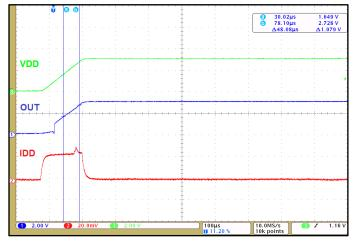
Figure 3. Power-On Time for Push-pull Output
