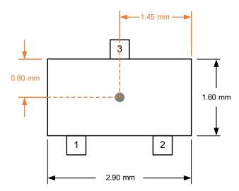
Figure 15. XtremeSense TMR Sensor Location for CT812x products in 3-lead SOT23 Package
