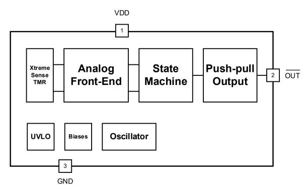
Figure 1. CT8122 with Push-pull Output Block Diagram for 3-lead SOT23 Package
