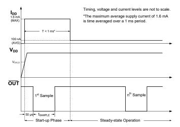
Figure 12. CT812x Power-On Timing Diagram
