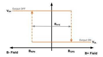
Figure 13. CT812x Output Behavior vs. Magnetic Field
