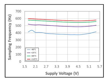
Figure 8. Sampling Frequency vs. Supply Voltage vs. Temperature
