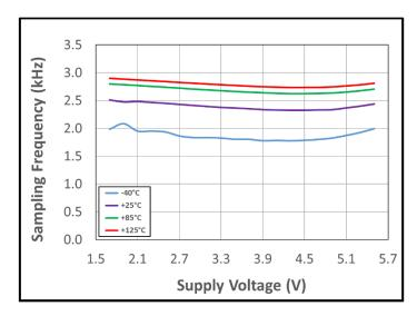
Figure 11. Sampling Frequency vs. Supply Voltage vs. Temperature
