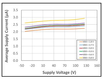
Figure 7. Average Supply Current vs. Temperature vs. Supply Voltage
