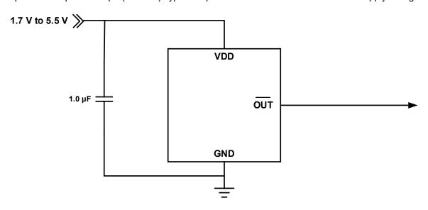
Figure 14. CT8122 Application Block Diagram
