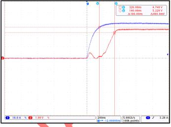
Figure 8. CT425 Response Time;  $I_P = 30 A_{PK}$  and  $C_L = 220 pF$  (Blue = lccc, Red = V<sub>OUT</sub>)
