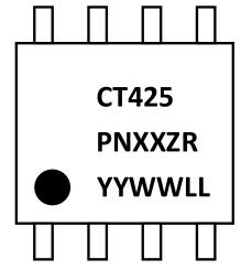
Figure 31. CT425 Device Marking for 8-lead Package
