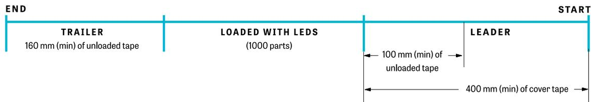
Each reel includes a leader and trailer section that is not loaded with LEDs.
