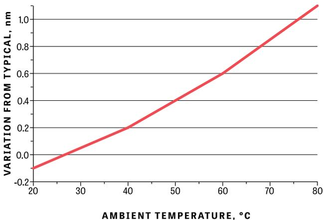
Test Conditions: Forward Voltage ( $I_f$ ) = 500 mA CW Operation
