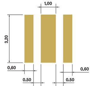
All dimensions are in millimeters. Unless noted otherwise, all dimensions have a tolerance of  $\pm 0.05$  mm.
