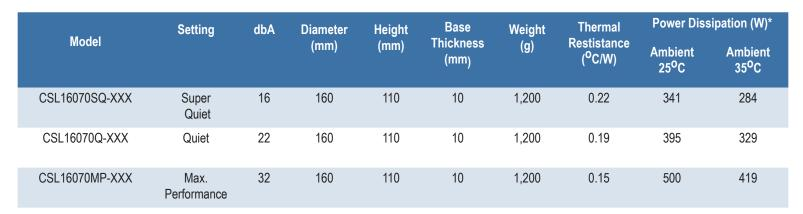
To select the heatsink part # for your light engine, go to pages 21 to 26 and replace the suffix '-XXX' with the suffix in the Selection Matrix.
