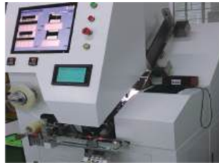
3 in 1 Auto inspection machine (Flatness/ Visual/ Taping)
