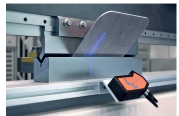
3D angle measurement during die pressing
