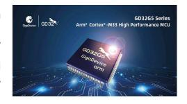
The GD32G5 series MCUs are equipped with 256KB to 512KB of embedded Flash memory, supporting the dual-bank Flash feature, and 128KB of SRAM, which includes 32KB Tightly Coupled Memory RAM (TCMRAM) for zero-wait execution of critical instructions and data. Additionally, they feature high-speed cache memory, with up to 2KB I-Cache and 512B D-Cache, further boosting core processing performance.
