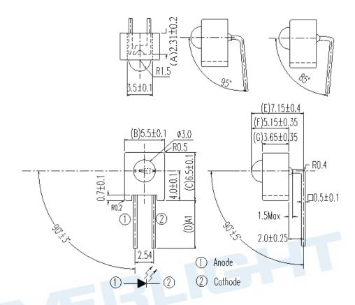
Note: Tolerances unless dimensions ±0.25mm
