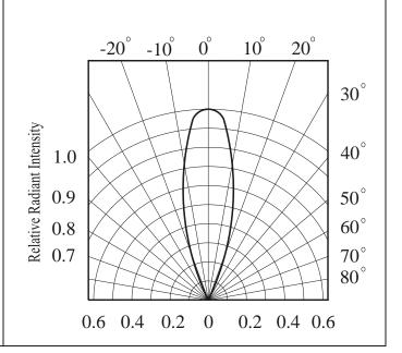
Relative Radiant Intensity vs. Angular Displacement
