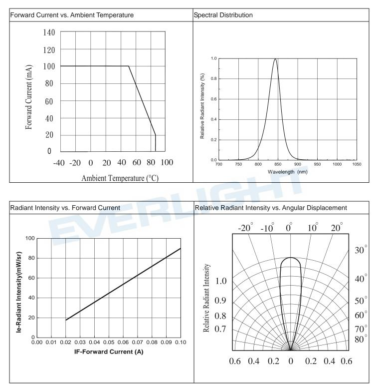
DATASHEET 3mm Infrared LED HIR204/H0
