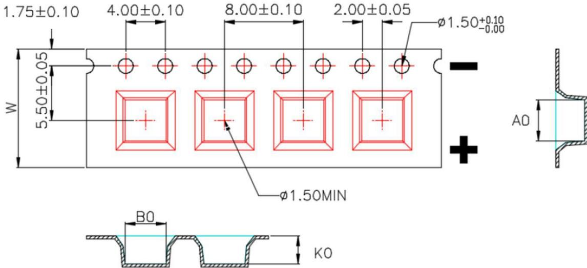
1. 10 sprocket hole pitch cumulative tolerance  $\pm 0.20$ .
