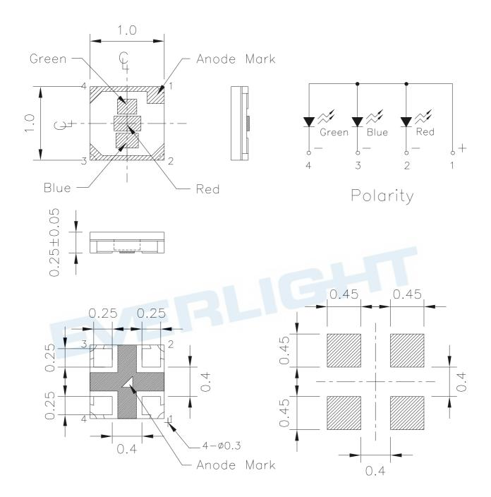
Note: Tolerances unless mentioned ±0.1mm. Unit = mm Suggested pad dimension is just for reference only.
