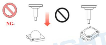
3. When using tweezers, prevent excessive stress form being applied to the LEDs; otherwise, the resin surfaces might be damaged, chipped, detached from the packages and the LED packages might be deformed. What is worse, the bonding wires might break up, resulting in no light emission. If necessary pick up by the package so as not to touch the encapsulating resin surface.
