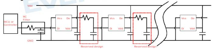
Note1: RC Filter and R1 must be added or reserved on the board for better waveform of signals in different applications.
