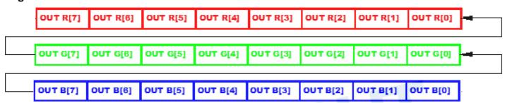
The single wire data transfer protocol supports 24-bit data for each LED RGB display data refresh. B1414IC receives 24-bit data and passes the remaining data to next LED. The 24-bit data consist of red, green and blue data, each with 8-bit width, and are transferred with MSB first.
