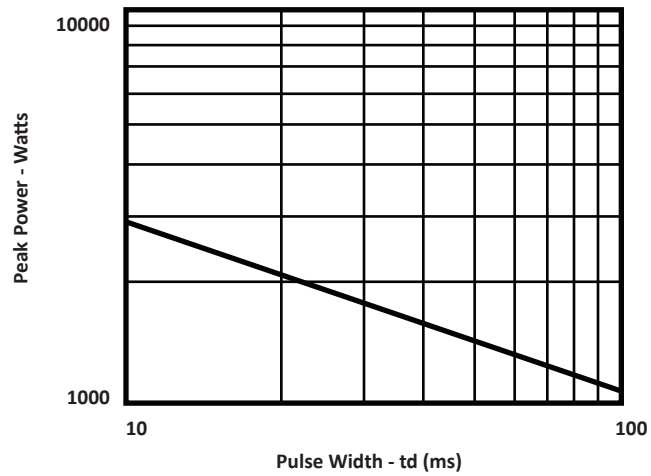
FIGURE 4 PEAK PULSE POWER RATING CURVE
