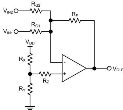
$$R_{VIN-} = \frac{1}{\frac{1}{R_{G1}} + \frac{1}{R_{G2}} + \frac{1}{R_F}}, R_{VIN-} = \text{total resistance at the inverting input.}$$
